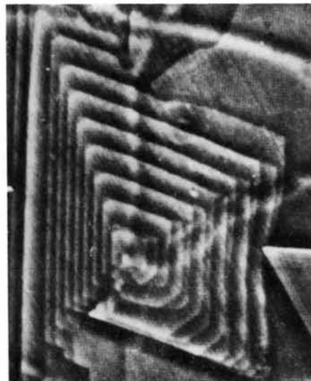
Fig. 3. Interlaced pattern due to growth round a half dislocation in crystal of the \alpha -form of n -alcohols ( 1600\times ).
